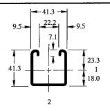
Wt/100 Ft:189 Lbs (281 kg/100 m) Allowable Moment 5,070 In-Lbs (570 N•m) 12 Gauge Nominal Thickness .105" (2.7mm)
