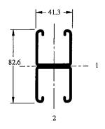
Wt/100 Ft: 378 Lbs (562 kg/100 m) Allowable Moment 14,360 In-Lbs (1,620 Nem) 12 Gauge Nominal Thickness .105" (2.7mm)
