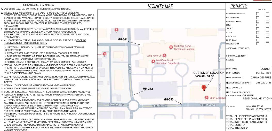
NARRATIVE:THIS PROJECT WILL PROVIDE CMS SERVICE TO 1450 5TH ST SE. EXISTING 24 STUB CABLE FROM POF\_MH-341 TO MH-341 IN EXISTING CONDUIT. EXISTING 24 FIBER CABLE FROM MH-341 TO MH-342 IN EXISTING CONDUIT. EXISTING 24 FIBER CABLE FROM MH-350 TO CUSTOMER MPOP PASSING THROUGH HH-1450 IN EXISTING CONDUIT.
