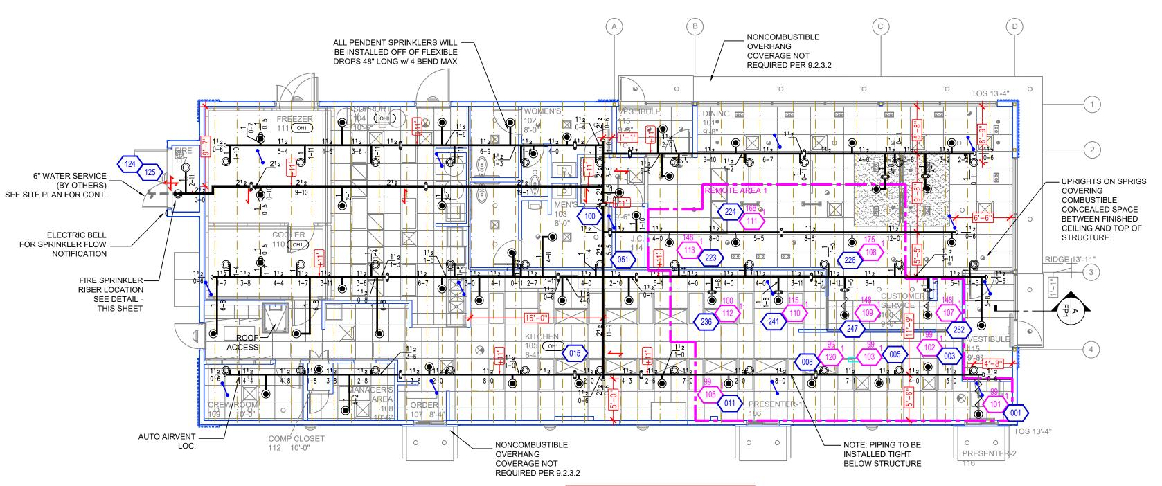
Design Area #: 1 HAZARD: **OH-1** Zone: **1** System Type: **WET** Location: KITCHEN 105 Flowing Outlets: 12 Density: 0.15 Remote Area: 900 Flow: **452.3** gpm @ **35** psi Calculation Safety: 7.1 psi Includes **250** gpm Hose allowance NOTE: AREA REDUCED BY 40% TO 900SF PER 19.3.3.2.3
