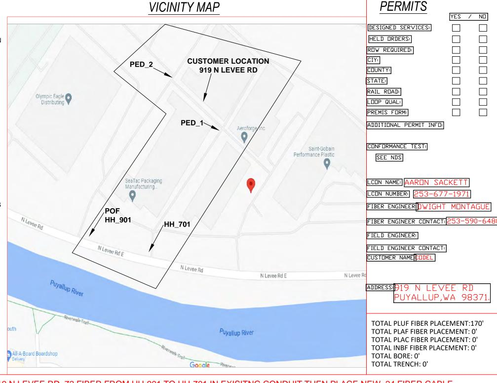
NARRATIVE: THIS PROJECT WILL PROVIDE CDFS SERVICE TO 919 N LEVEE RD. 72 FIBER FROM HH-901 TO HH-701 IN EXISITNG CONDUIT. THEN PLACE NEW 24 FIBER CABLE FROM HH 701 TO CUSTOMER MPOP THROUGH PED'S IN EXISITNG CONDUIT.
