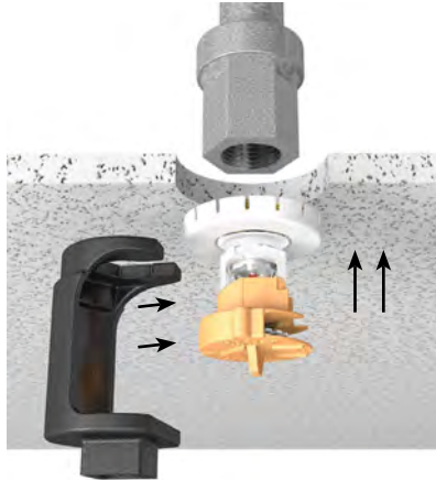
Figure 3: Recessed Installation (with Recessed Socket Wrench)
