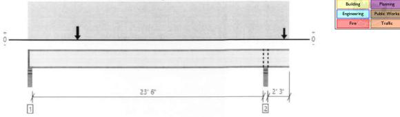
All locations are measured from the outside face of left support (or left cantilever end). All dimensions are horizontal.
