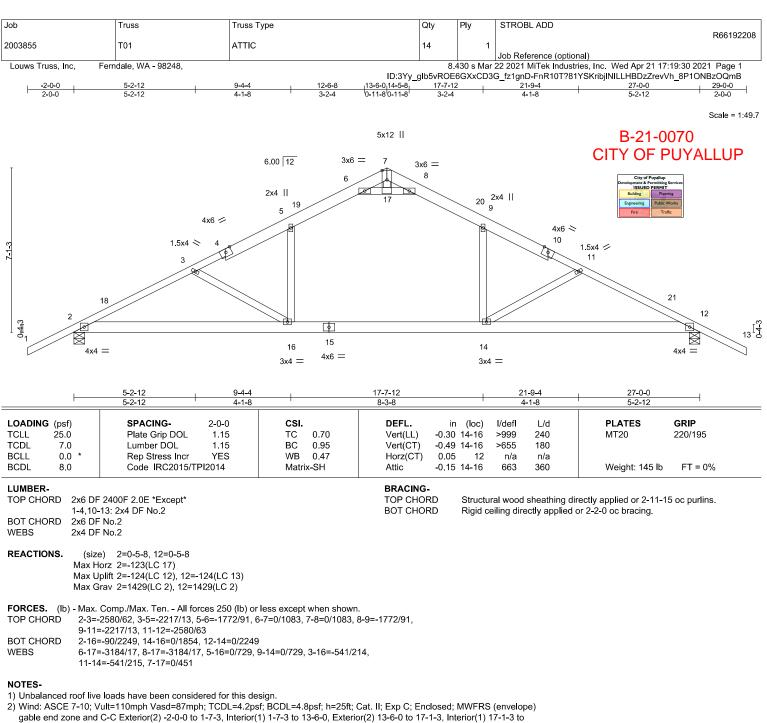
gable end zone and C-C Exterior(2) -2-0-0 to 1-7-3, Interior(1) 1-7-3 to 13-6-0, Exterior(2) 13-6-0 to 17-1-3, Interior(1) 17-1-3 to 29-0-0 zone; cantilever left and right exposed; end vertical left and right exposed; C-C for members and forces & MWFRS for reactions shown; Lumber DOL=1.60 plate grip DOL=1.60
