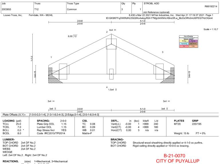
Max Horz 1=-21(LC 17) Max Uplift 1=-24(LC 12), 3=-24(LC 13) Max Grav 1=145(LC 1), 3=145(LC 1)
