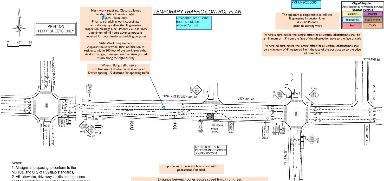
2. All sidewalks, driveways, exits and egresses shall be completely clear unless otherwise indicated. 3. Channelizing devices are 28" traffic cones. Use traffic drums (barrels) with steady burning Type C lights on all State State Routes and Hwys. 4. Sign size can be a minimum of 36" x 36" and shall not obstruct pedestrian access.
