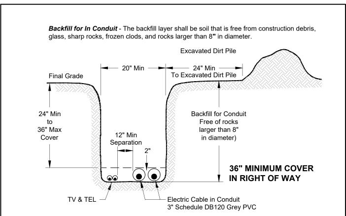
CUSTOMER-SUPPLIED TRENCH FOR SECONDARY DIST. (P01 TO HH1) SCALE: NONE
