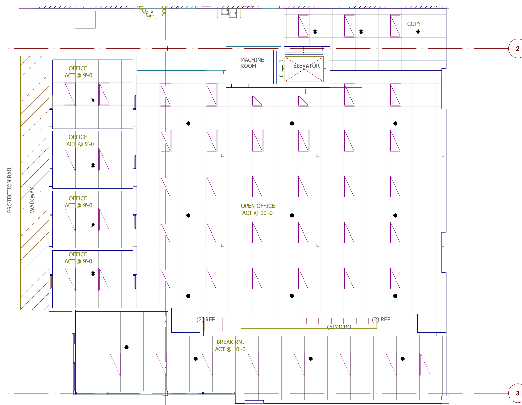
UNDER MEZZANINE ADDITION - REFLECTED CEILING PLAN
