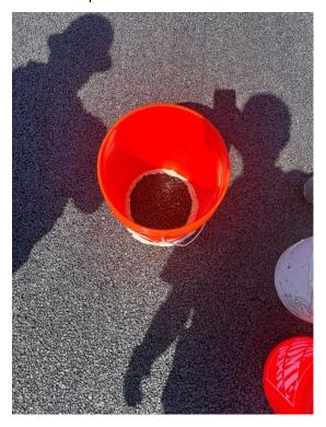
The pervious asphalt yields an approximate infiltration rate of 540 in/hr based on the results/findings of the infiltration test performed on the pervious asphalt installed with this project.
