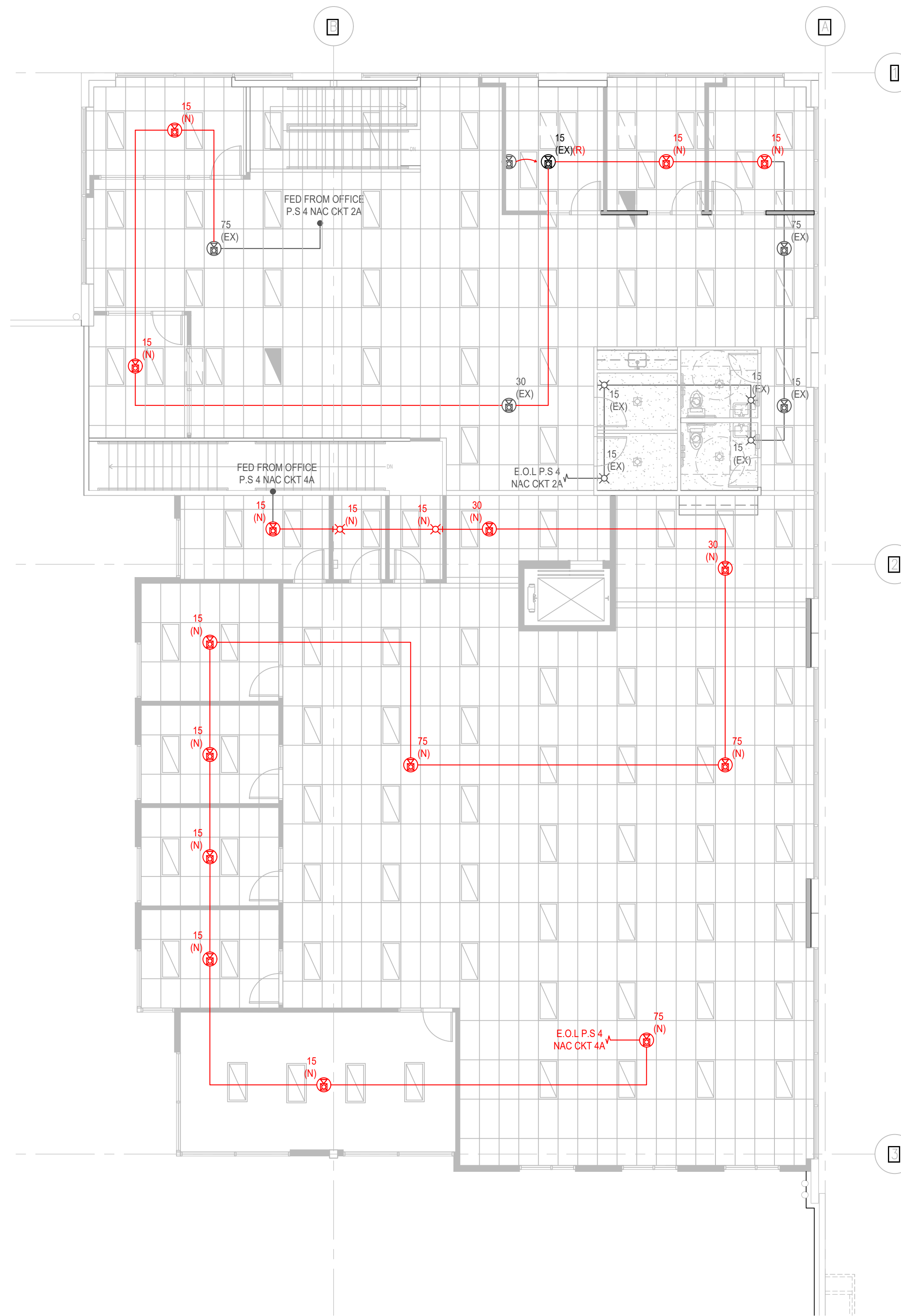
2 FIRE ALARM OFFICE 2ND FLOOR NAC LAYOUT 1/8"=1'-0"
