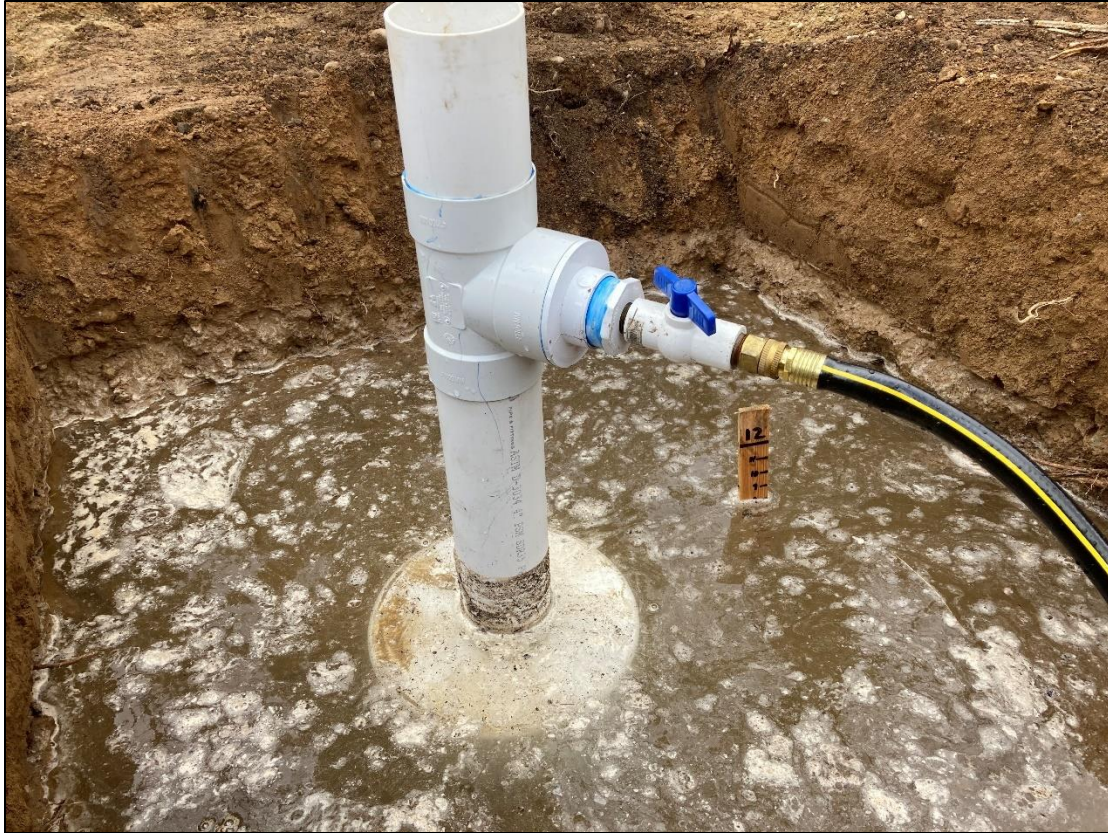
Figure 2: Infiltration Test in Progress
