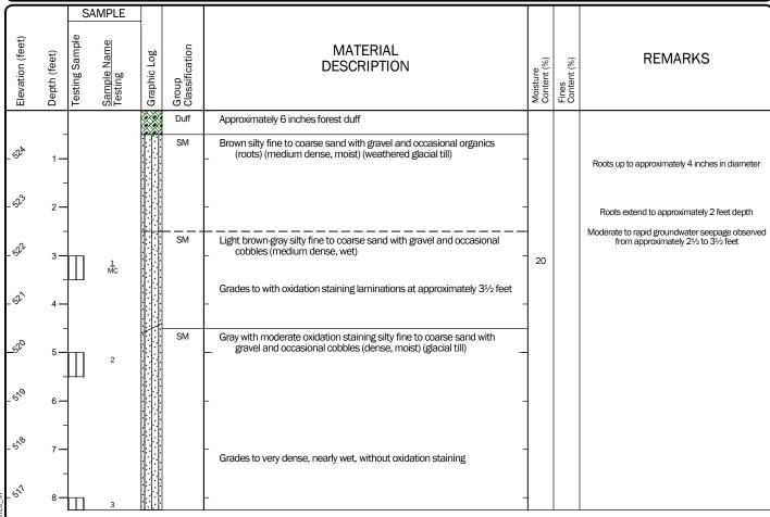
Notes: See Figure A-1 for explanation of symbols. The depths on the test pit logs are based on an average of measurements across the test pit and should be considered accurate to ½ foot. Coordinates Data Source: Horizontal approximated based on Google Earth. Vertical approximated based on Topographic Survey.
