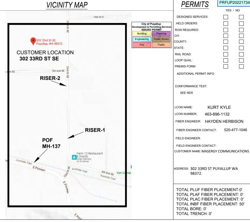
NARRATIVE: THIS PROJECT WILL PROVIDE CDFS SERVICE TO 302 33RD ST SE. PUSH COUNTS ON EXISTING 48 FIBER CABLE FROM POF MH-137 TO POLE-1 PASSING THROUGH EXISTING PED IN EXISTING CONDUIT. PUSH COUNTS ON EXISTING 48 FIBER CABLE FROM POLE-1 TO POLE-2 TO CUSTOMER MPOP IN EXISTING AERIAL ROUTE.
