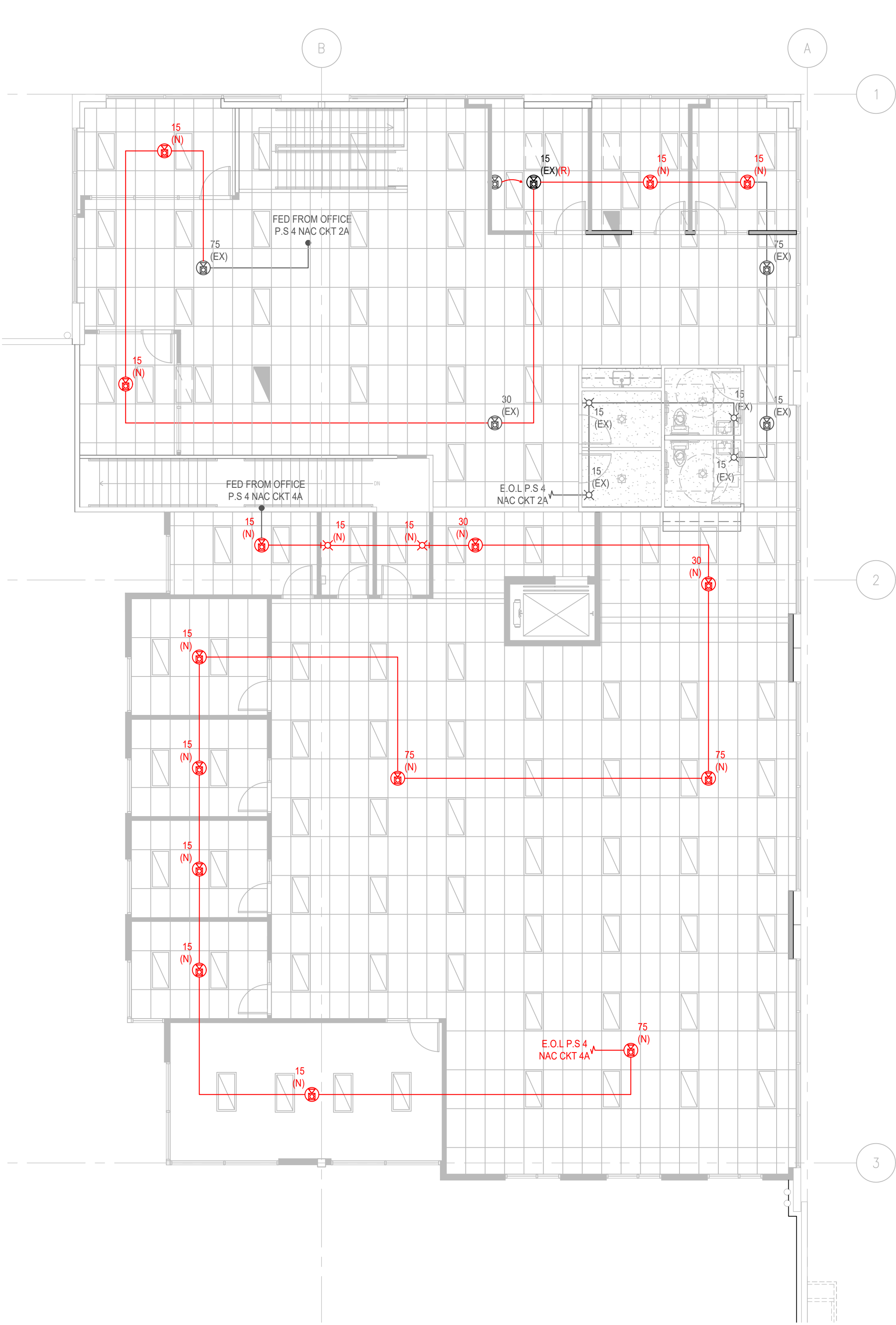
2 FIRE ALARM OFFICE 2ND FLOOR NAC LAYOUT 1/8"=1'-0"
