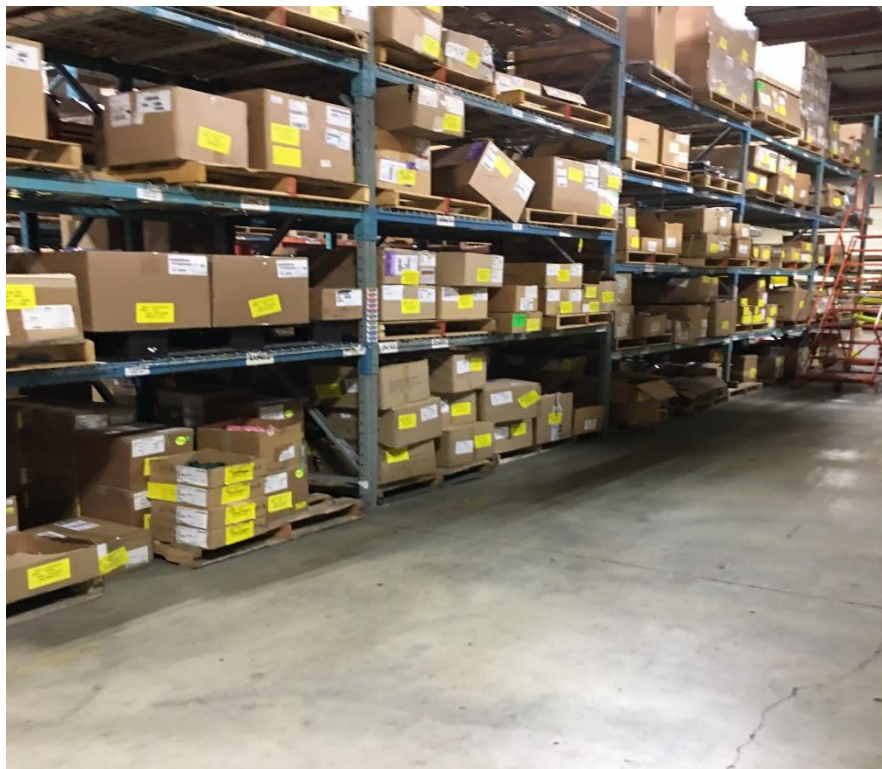
Picture 4 – Flue with Pallet Load
