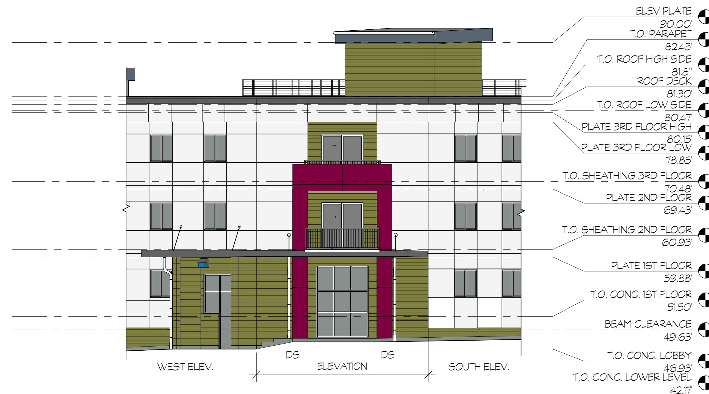
2 NORTH EXTERIOR ELEVATION A2.2 SCALE: 1/8" = 1'-0"
