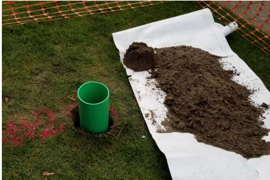
Photo 2: Test pit 2 infiltration testing.
