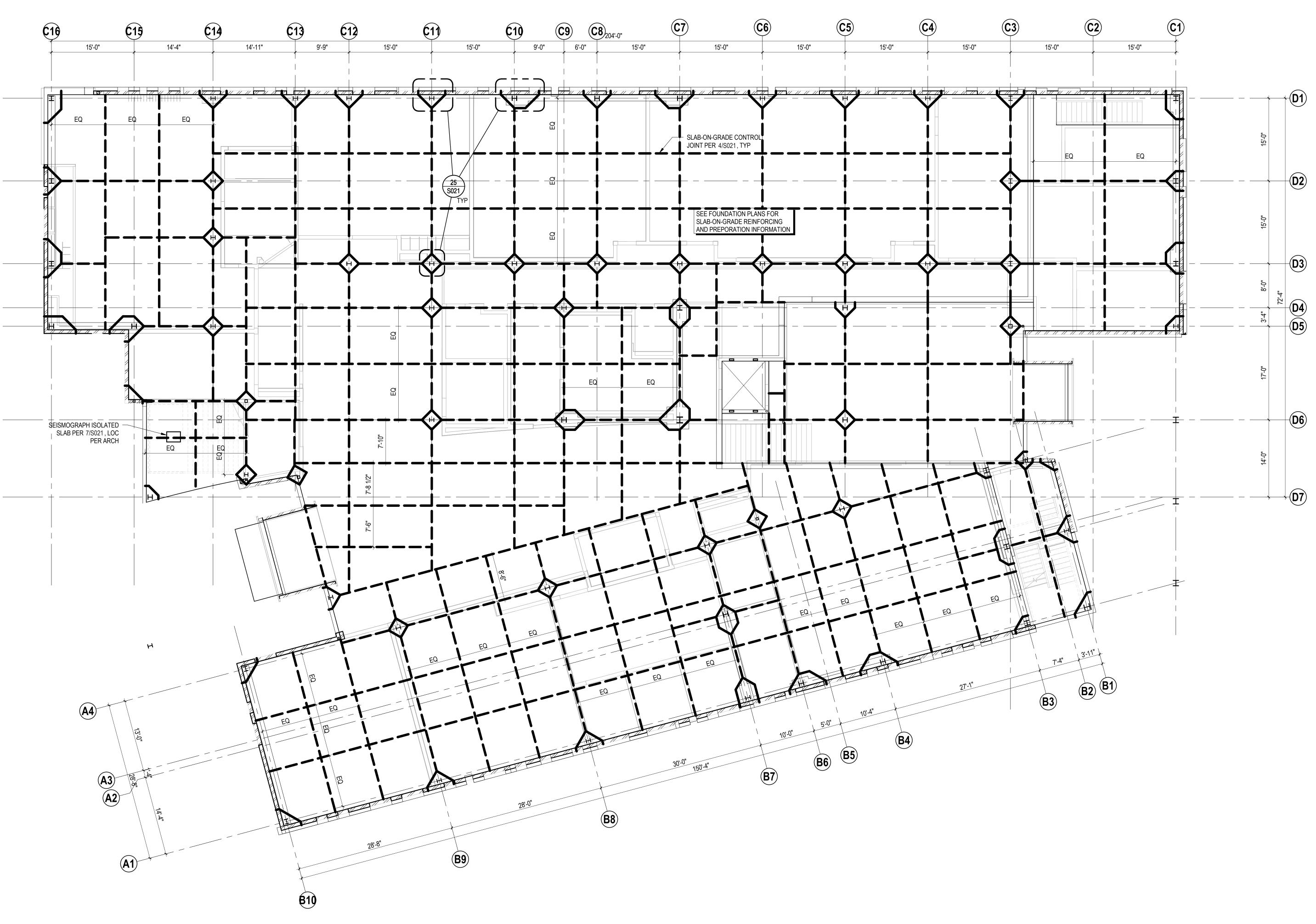
SLAB CONTROL JOINT PLAN - SLAB-ON-GRADE SCALE: 1/8" = 1'-0"
