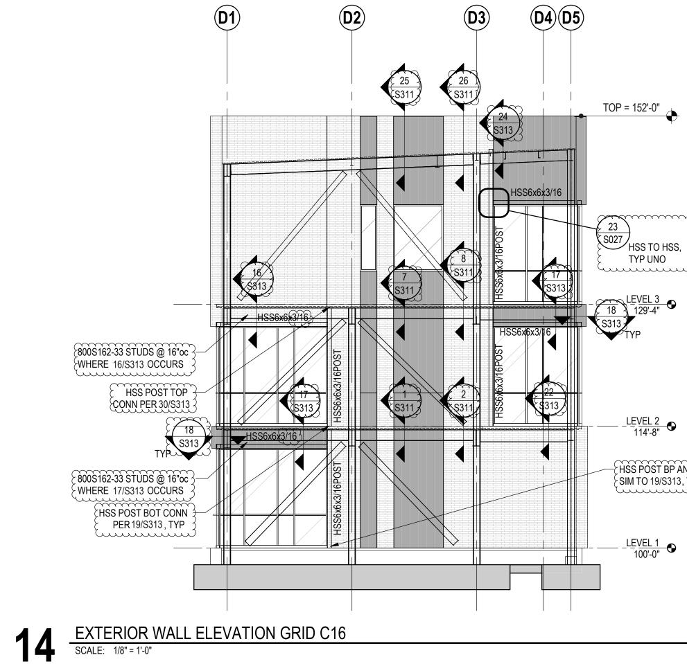
EXTERIOR METAL STUD WALL NOTES: 1. FOR TYPICAL METAL STUD DETAILS SEE SHEETS S023 & S024
