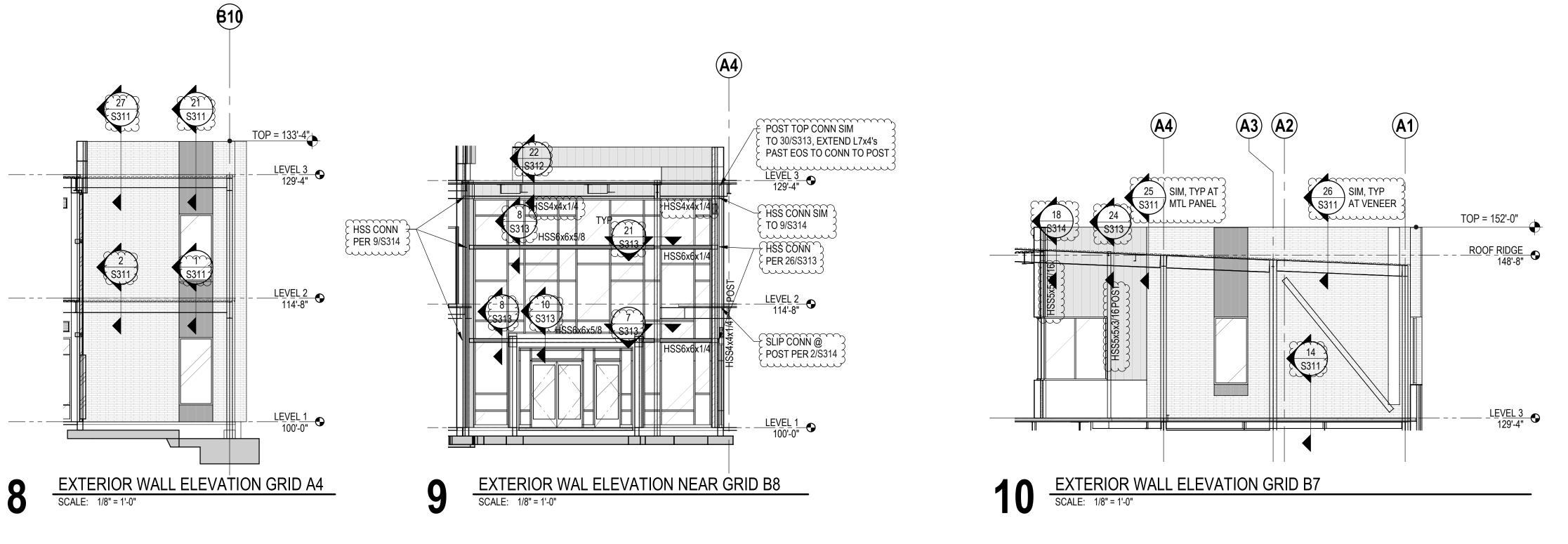
EXTERIOR METAL STUD WALL NOTES: 1. FOR TYPICAL METAL STUD DETAILS SEE SHEETS S023 & S024
