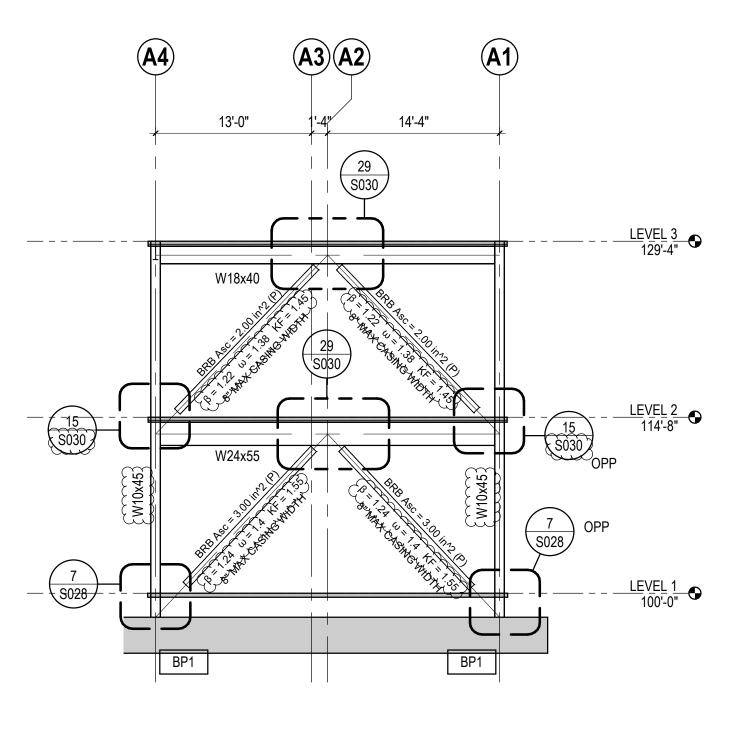
BRACE FRAME ELEVATION - GRID B10 SCALE: 1/8" = 1'-0"
