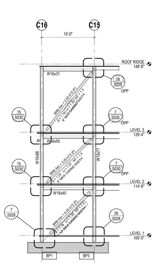
BRACE FRAME ELEVATION - GRID D5 SCALE: 1/8" = 1'-0"
