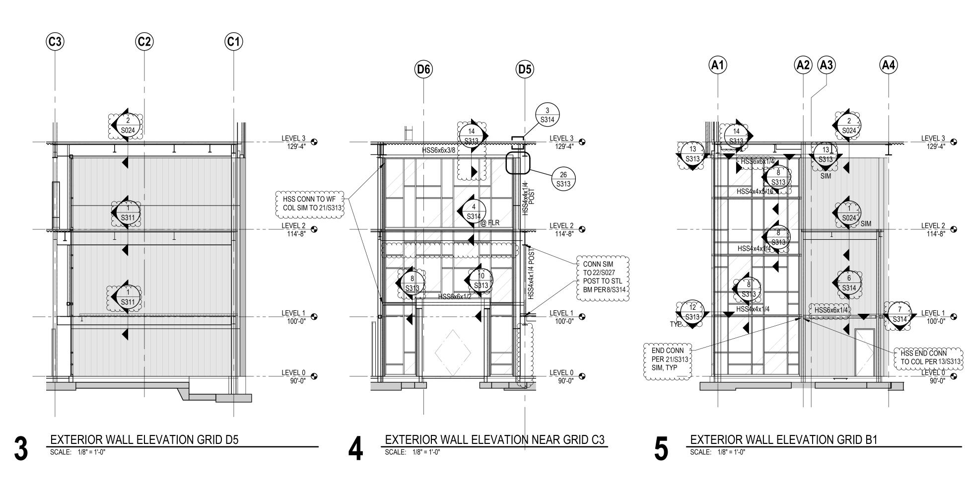
EXTERIOR METAL STUD WALL NOTES: 1. FOR TYPICAL METAL STUD DETAILS SEE SHEETS S023 & S024
