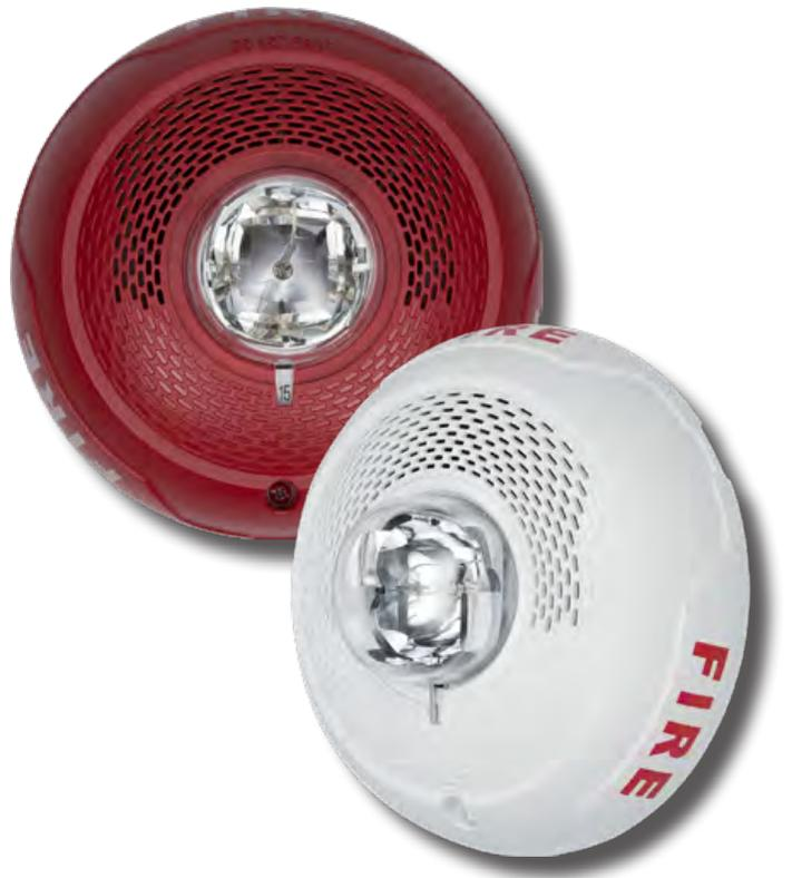
**System Sensor L-Series** of speakers and speaker strobes reduce costly ground faults using a plug-in design and universal mounting plate that allow the installer to pre-wire mounting plates, dress the wires, and confirm wiring continuity before plugging in the speakers. In addition, a protective plastic cover prevents nicked wires by covering exposed speaker components.
