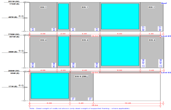
Shear Wall at Grid 1
