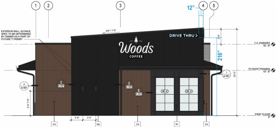
EXTERIOR ELEVATION - SOUTH
