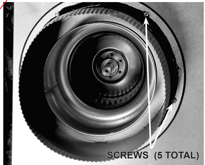
Figure 8F.4 Base Plate Fastened to Intake
