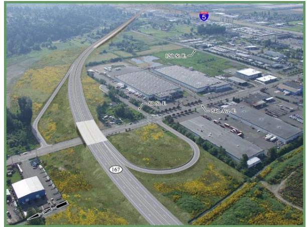
Visualization of the preferred Loop Ramp interchange option at 54th Avenue East
