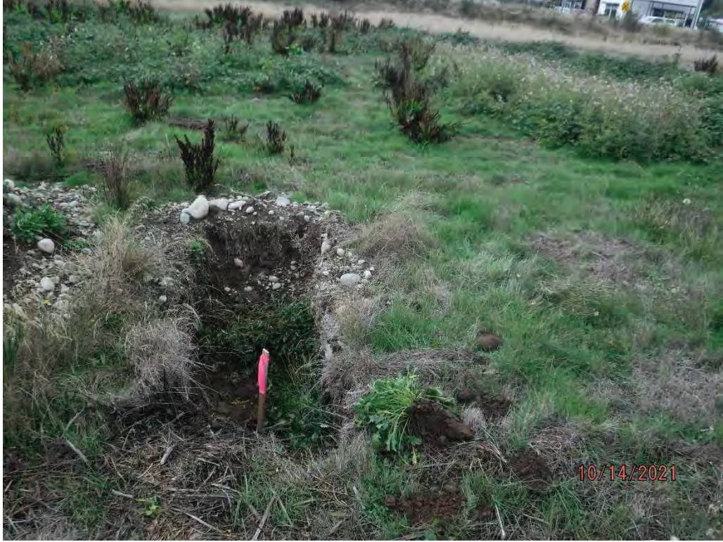
View of the depth of fill in the central portion of the project site – SP#3.
