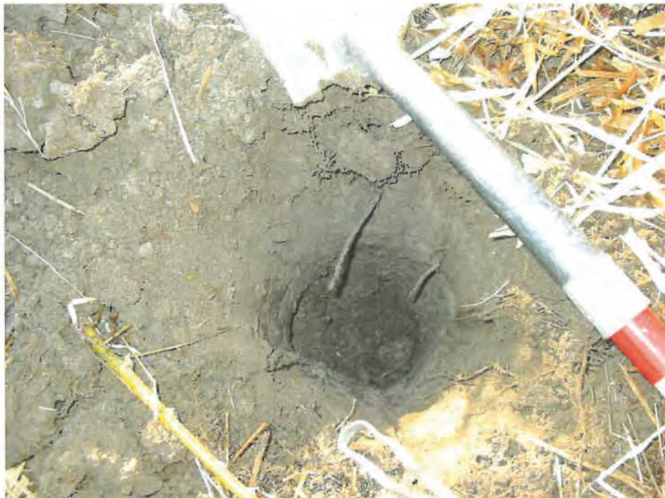
Photo #6: Looking down into the bottom of TP3 with no saturation or groundwater evident at this time in the lowest part of the old drainage ditch that had flowed along the eastern side of the project site. (IMG-020, 3/4/20)
