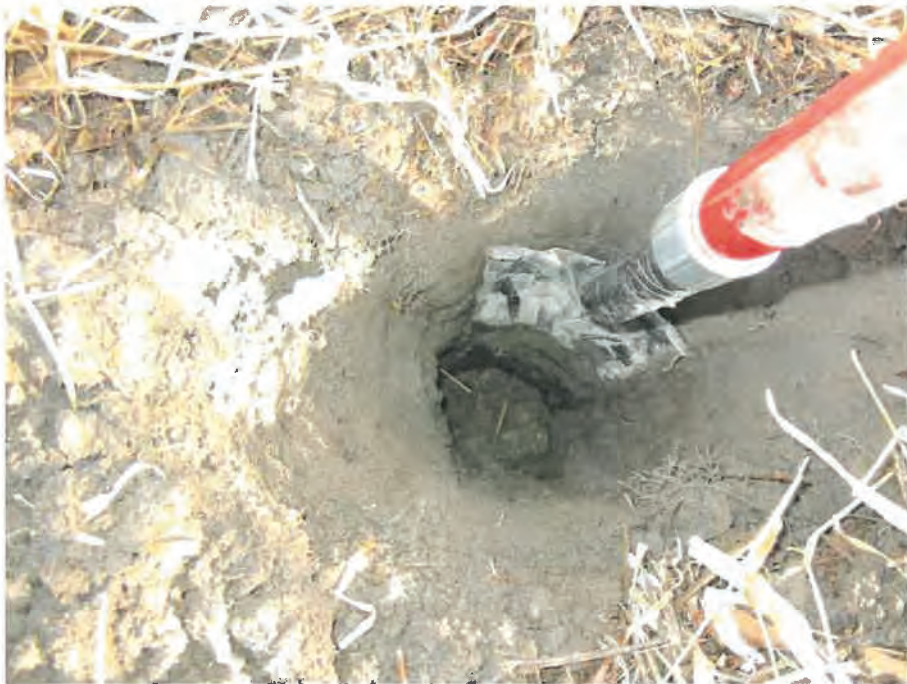
Photo #4: Looking down into the bottom of test hole at TP1 that has no seepage or groundwater evident at 24" deep. Note the soil color was also indicating non-wetland by field color indicators. (IMG-008, 3/4/20)
