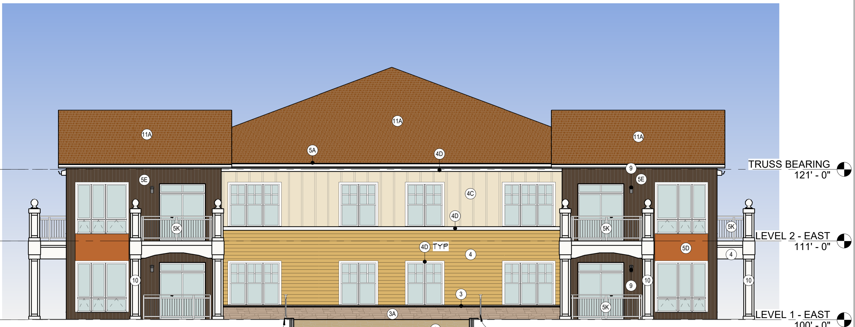
1 EXTERIOR ELEVATION - NORTH END A3.2-B/ 1/8" = 1'-0"
