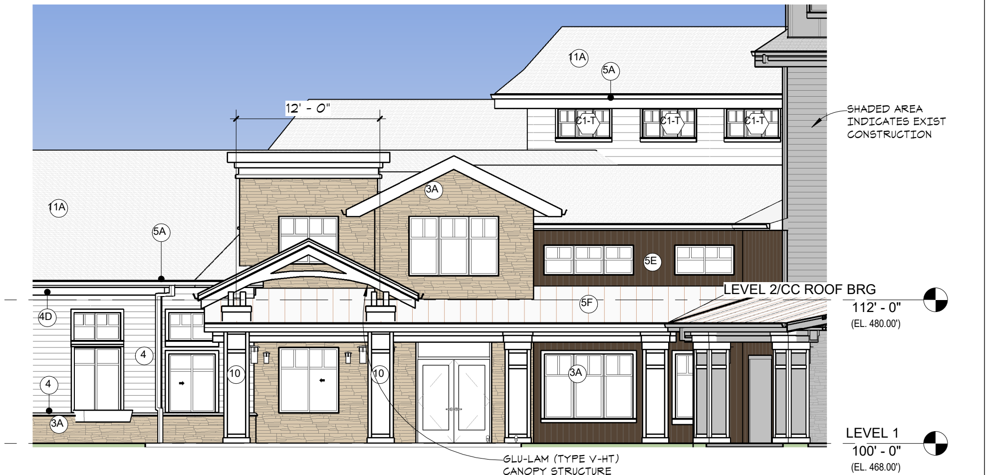
1 EXTERIOR ELEVATION - CC ENTRY A3.1 1/8" = 1'-0"
