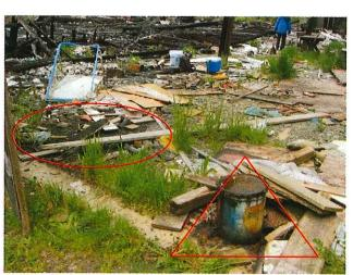
6. Leakage is visible around bottom of container, as well as a heavily stained area to the south (left)..
