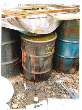
Sample location of S2-00-051011, in the stained area adjacent to a leaking drum in the SE corner of the drum group. Note the material hardened on the side of the drum and emanating from a hole now plugged.
