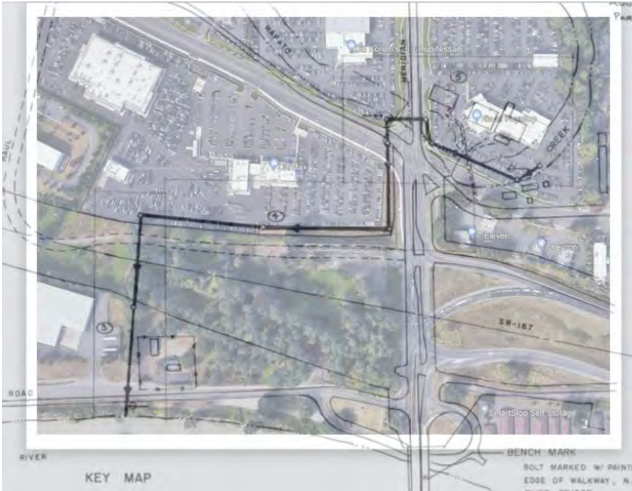
Figure 5. June 1, 1979 as-built overview for Wapato Creek Diversion approximate overlay on modern aerial. Lower image: Inlet (lower right) and outlet to Puyallup River (lower left) of the Wapato Diversion.
