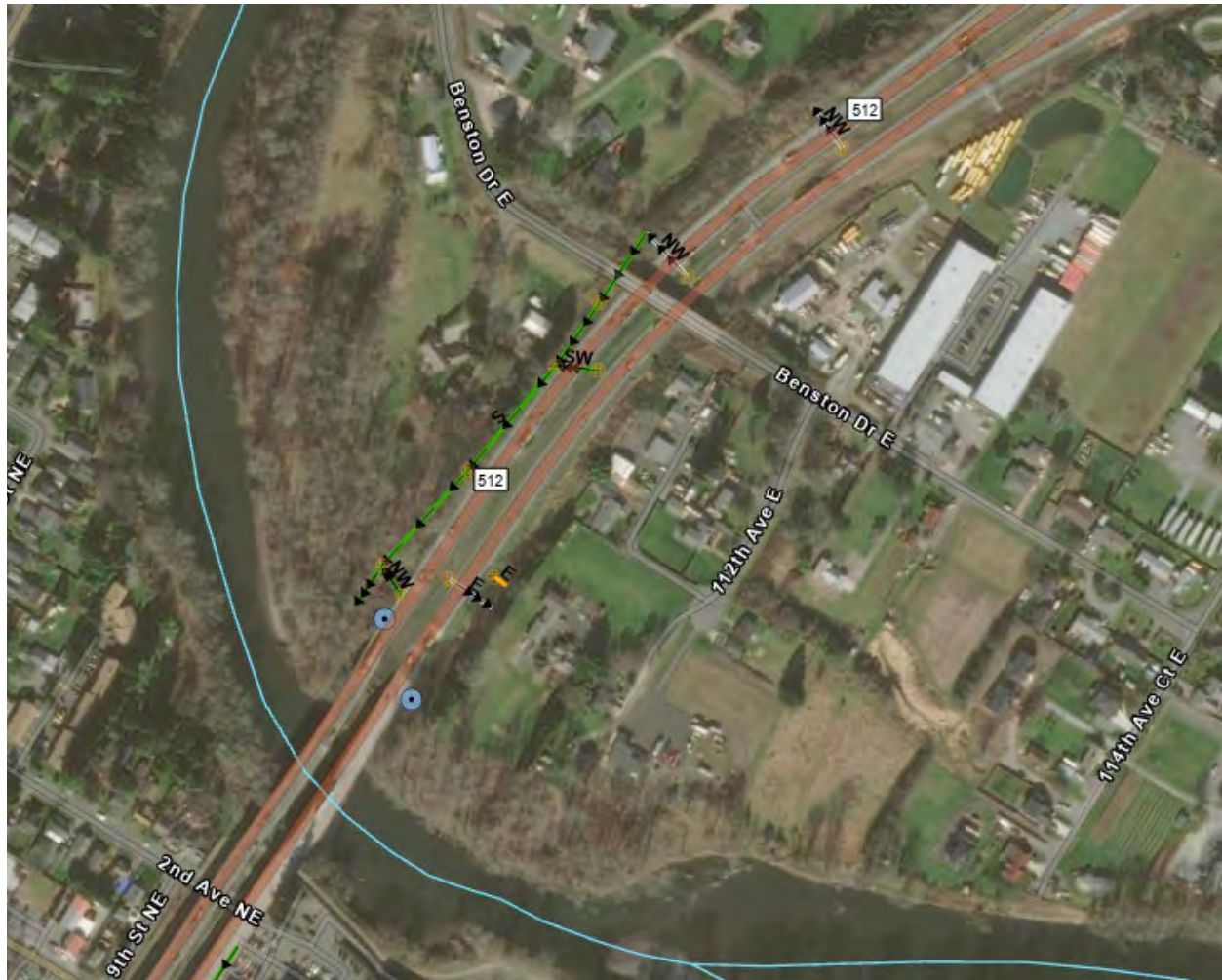
Figure 4. The other location of surface water discharge outlets (blue dots) from stormwater pipes empty onto elevated floodplain areas and may be outside of the 100-yr flood elevation. The flows are likely dispersed down sloped engineered channel or through uplands. This is a very limited drainage area from the median and road runoff.
