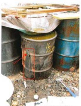
Sample location of \$2-00-051011, in the stained area adjacent to a leaking drum in the SE corner of the drum group. Note the material hardened on the side of the drum and emanating from a hole now plugged.
