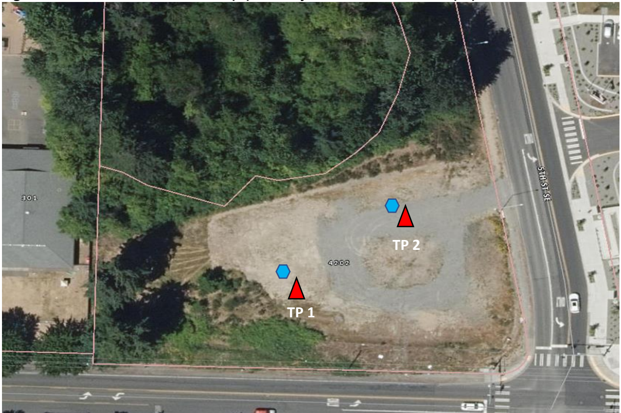
Figure 3: Lot-C Infiltration Test PIT (◈) and Adjacent observation PIT (▲) Locations
