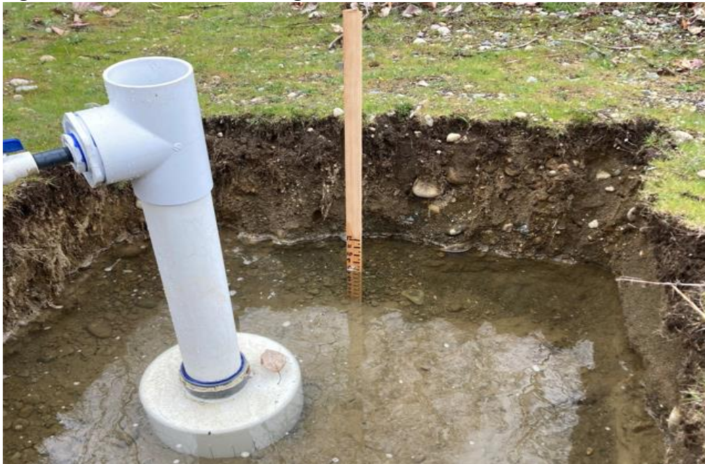
Figure 6: Infiltration Test in Progress PIT 1, Lot C
