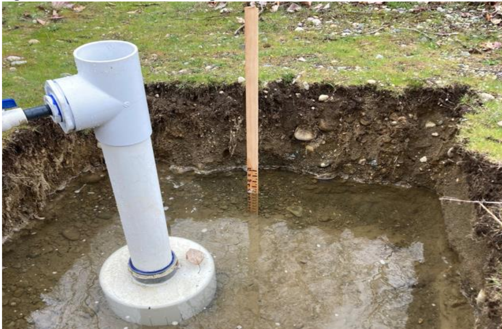
Figure 6: Infiltration Test in Progress PIT 1, Lot C
