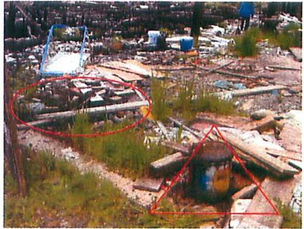
6. Leakage is visible around bottom of container, as well as a heavily stained area to the south (left)..
