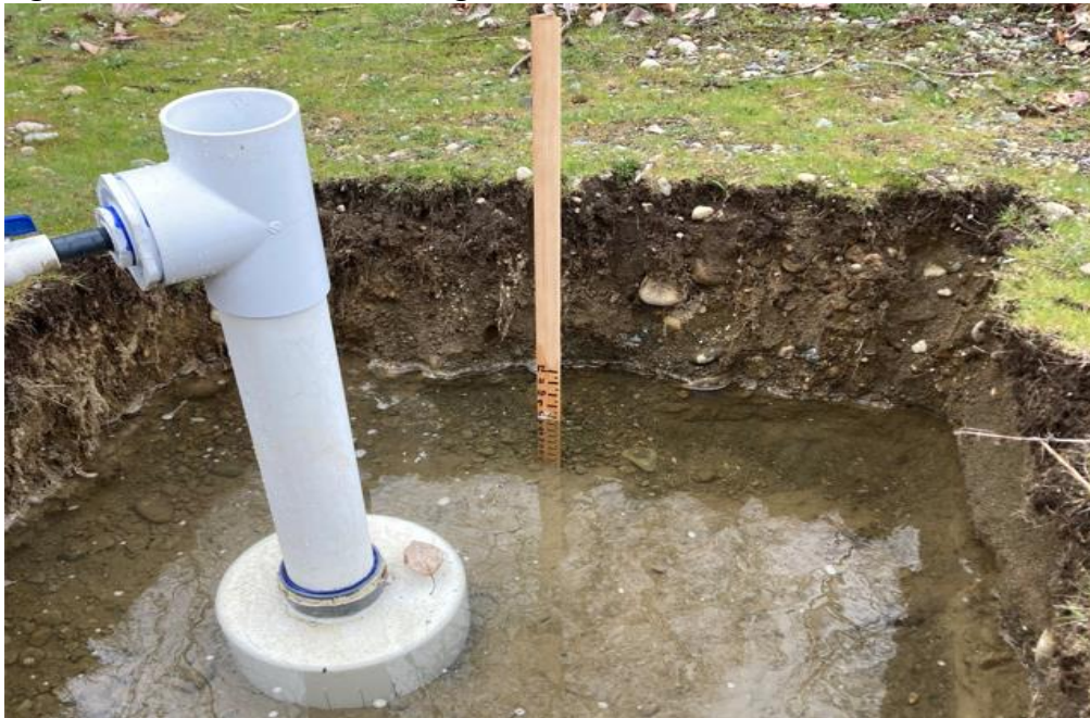
Figure 6: Infiltration Test in Progress PIT 1, Lot C
