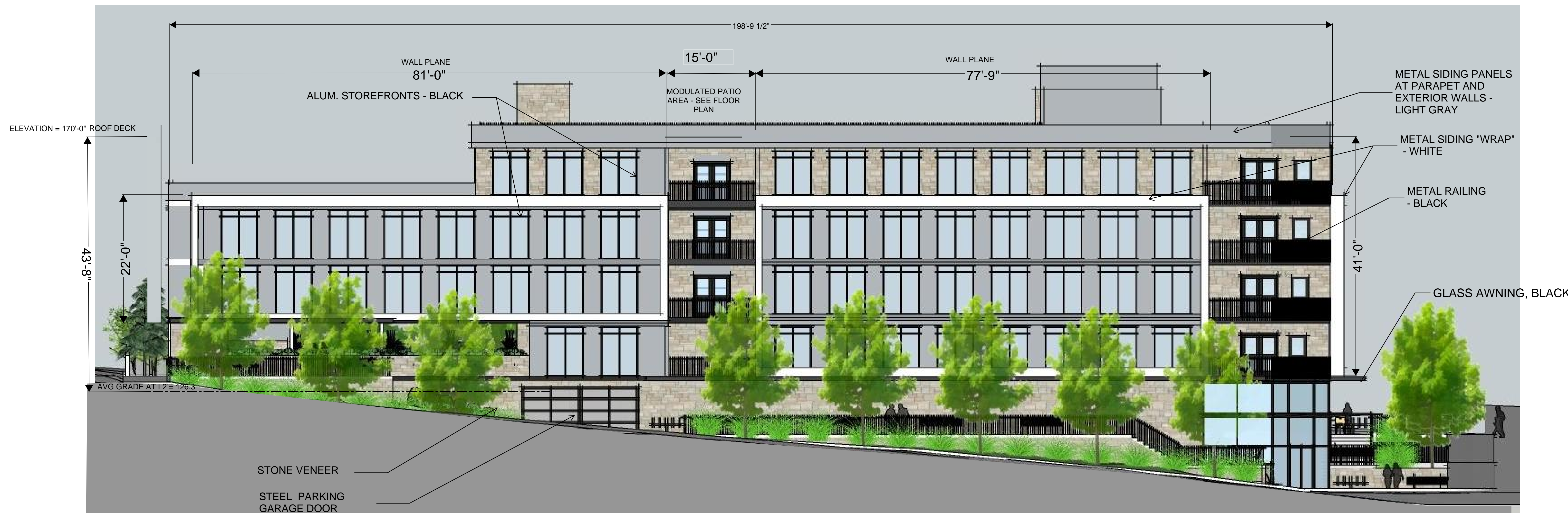
NORTH EXTERIOR ELEVATION
