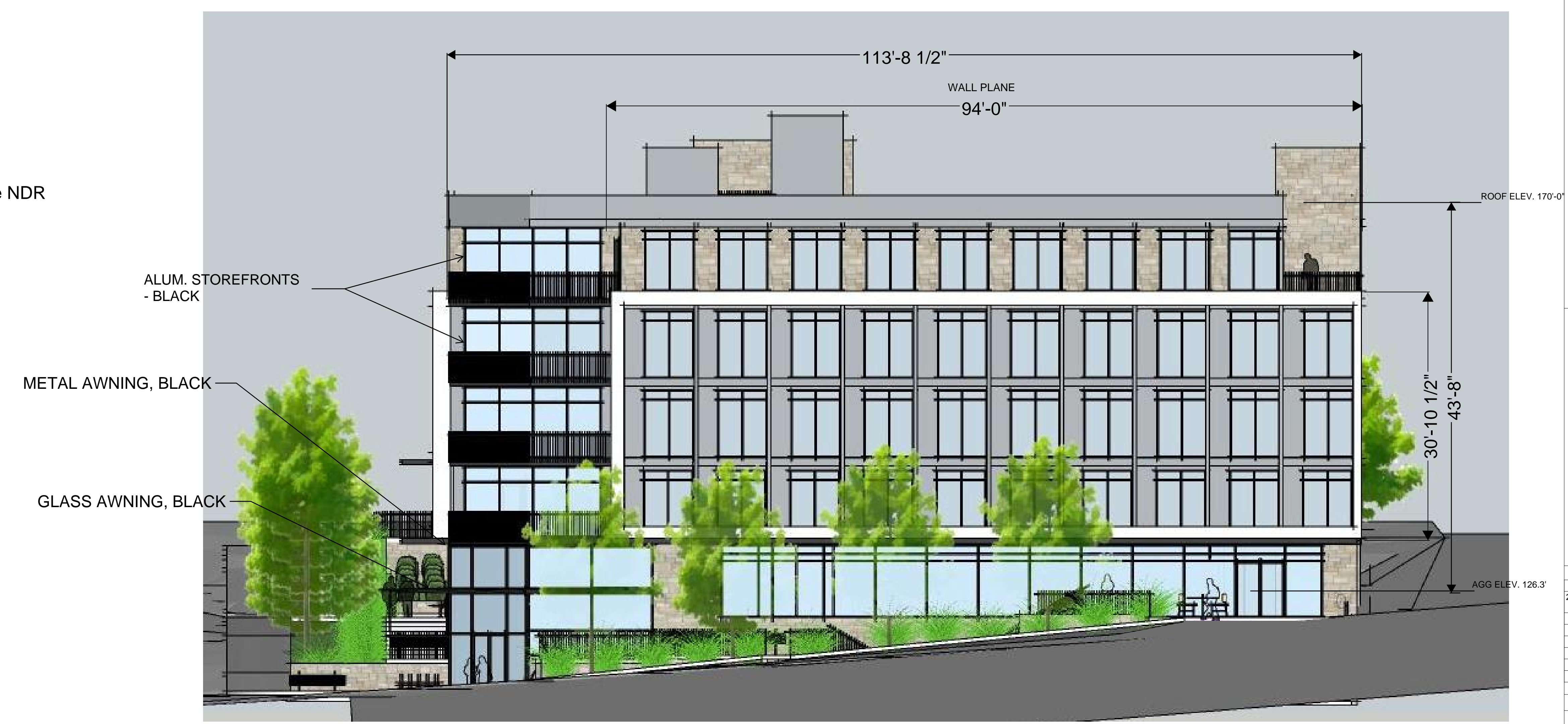
WEST EXTERIOR ELEVATION
