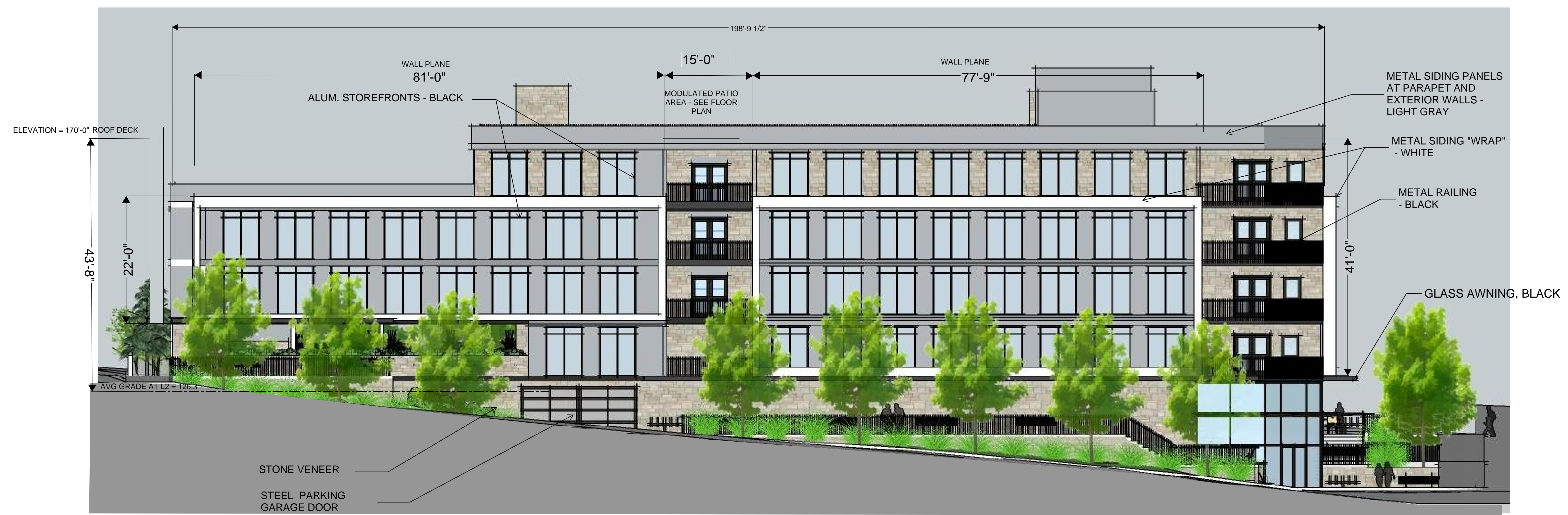
NORTH EXTERIOR ELEVATION
