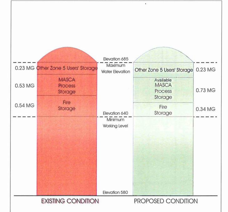
Tank has a storage capacity of 1.30 MG above hydraulic working grade of 640 feet.
