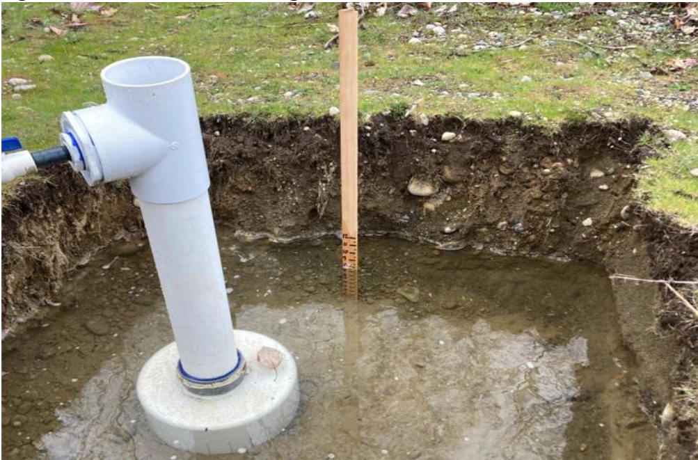
Figure 6: Infiltration Test in Progress PIT 1, Lot C
