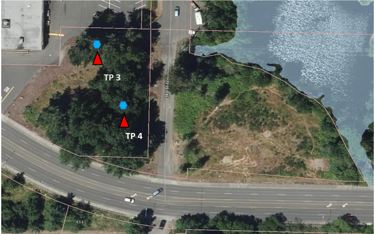
Figure 4: Lot-D Infiltration Test PIT (◈) and Adjacent observation PIT (▲) Locations
