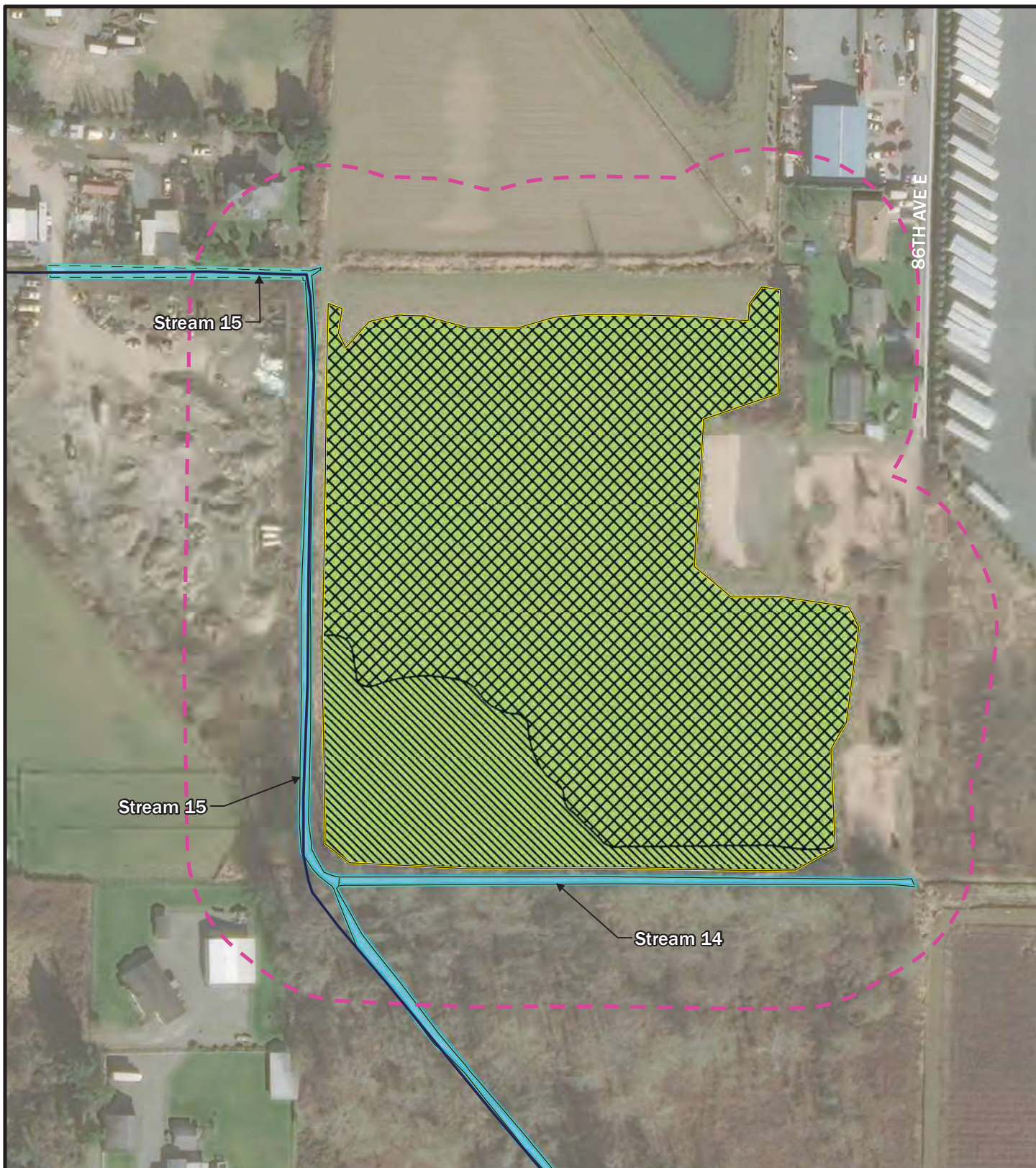
Figure D-40. Hydroperiod, 150-Foot Boundary, and Location of Outlets for Wetland 93.
