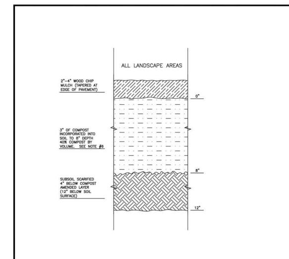
. ALL SOIL AREAS DISTURBED OR COMPACTED DURING CONSTRUCTION, AND NOT COVERED BY BUILDINGS OR PAVEMENT, SHALL BE AMENDED WITH COMPOST AS DESCRIBED BELOW.
