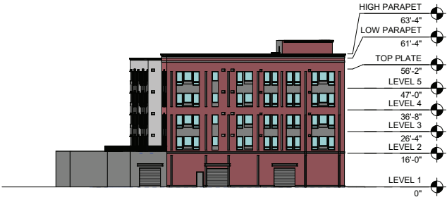
SOUTH ELEVATION - ALLEY FACING
