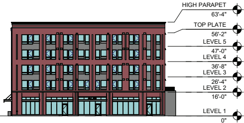
NORTH ELEVATION - STREET FACING
