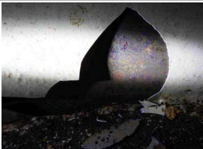
Lower Shell Large Coating Failure
