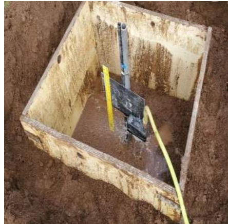
Test Pit Pre-soak at 12-inches
