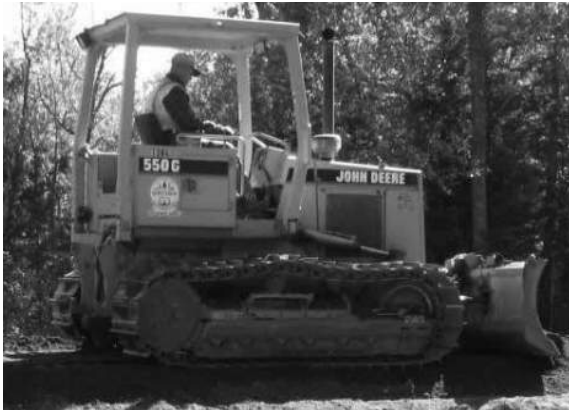
Examples of light, tracked, construction equipment used to place final cover over the pipe system.
