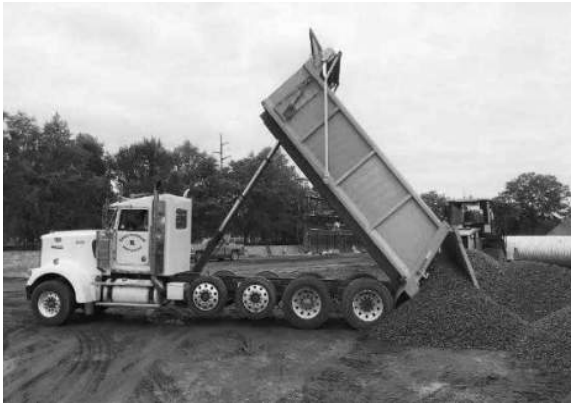
Examples of heavy construction equipment that may require additional minimal cover.
