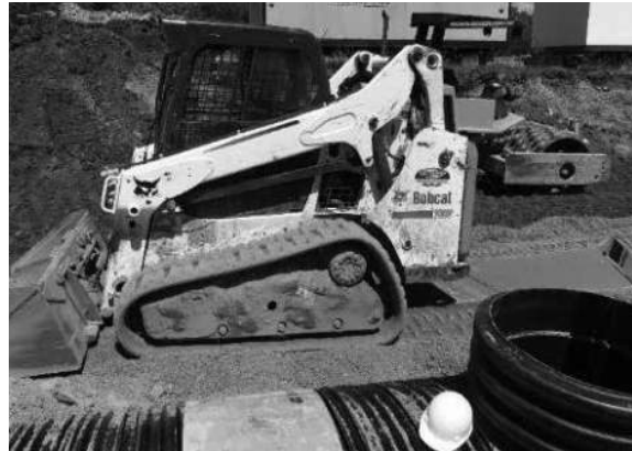
Examples of light, tracked, construction equipment used to place final cover over the pipe system.
