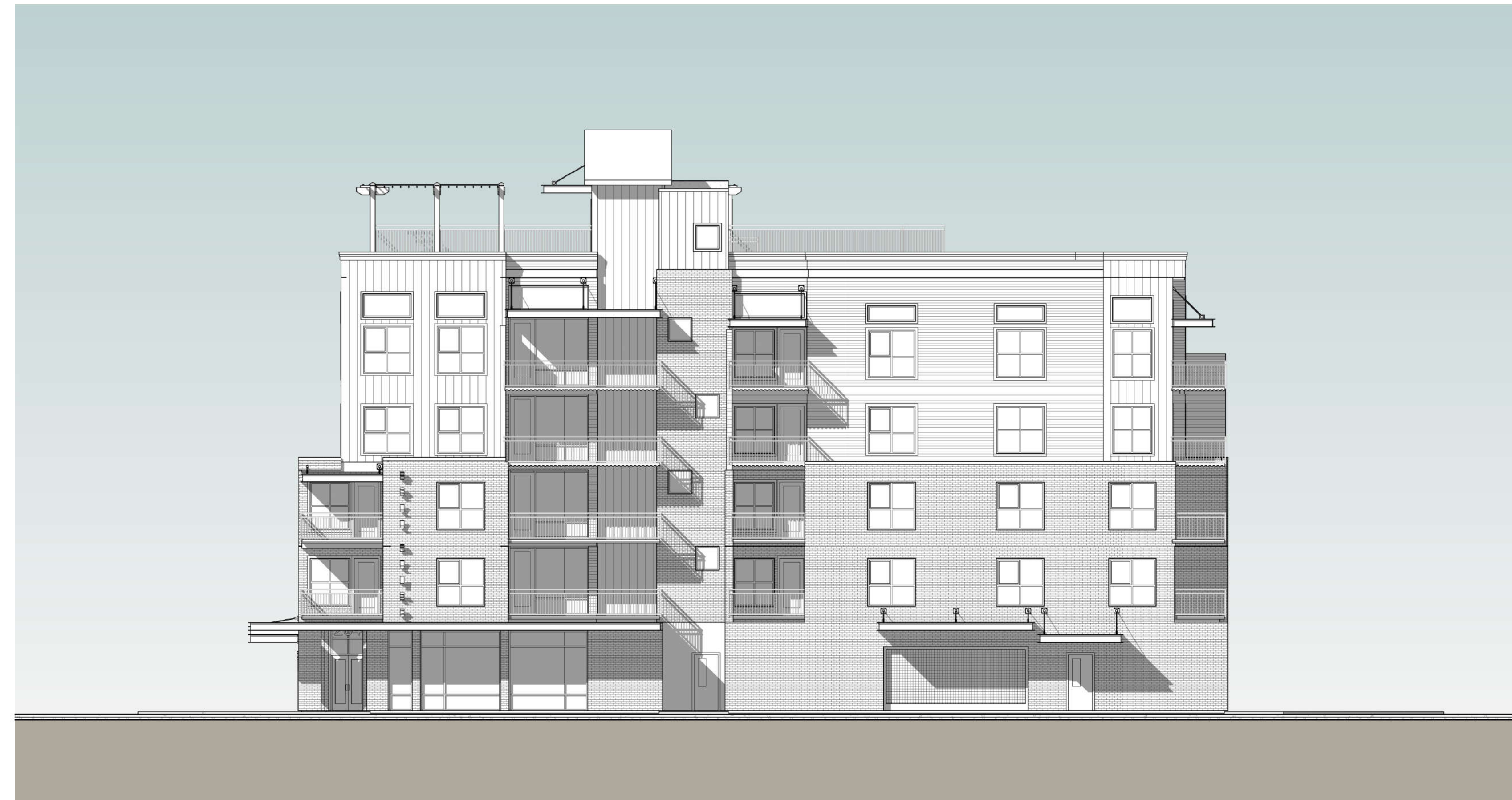
EAST ELEVATION - 4th Street SW 3/32" = 1'-0"
