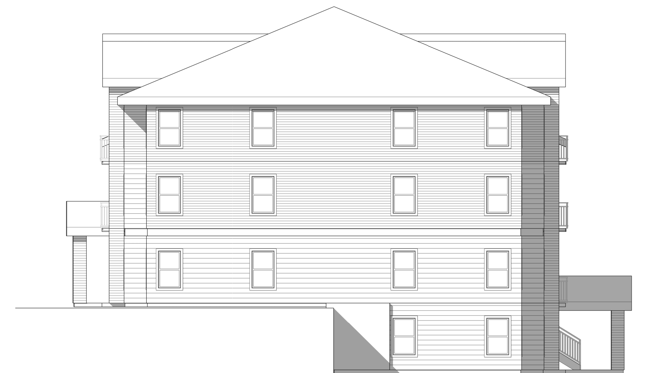
Building H - East Elevation / Side 1/8" = 1'-0"
