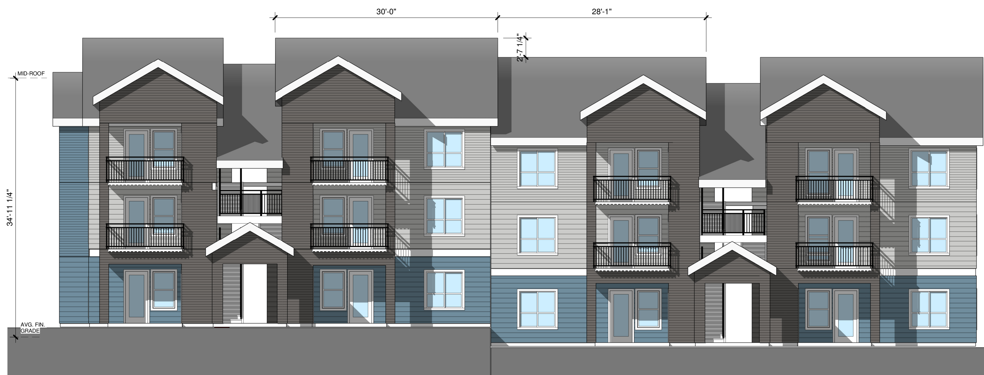
Building E - North Elevation / 27th Ave SE 1/8" = 1'-0"
