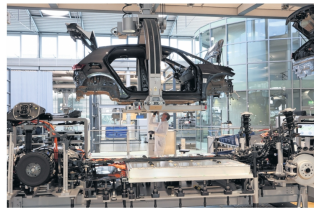
A worker prepares the undercarriage of a Volkswagen ID3 electric automobile for battery pack installation at the automaker's factory in Dresden, Germany.
