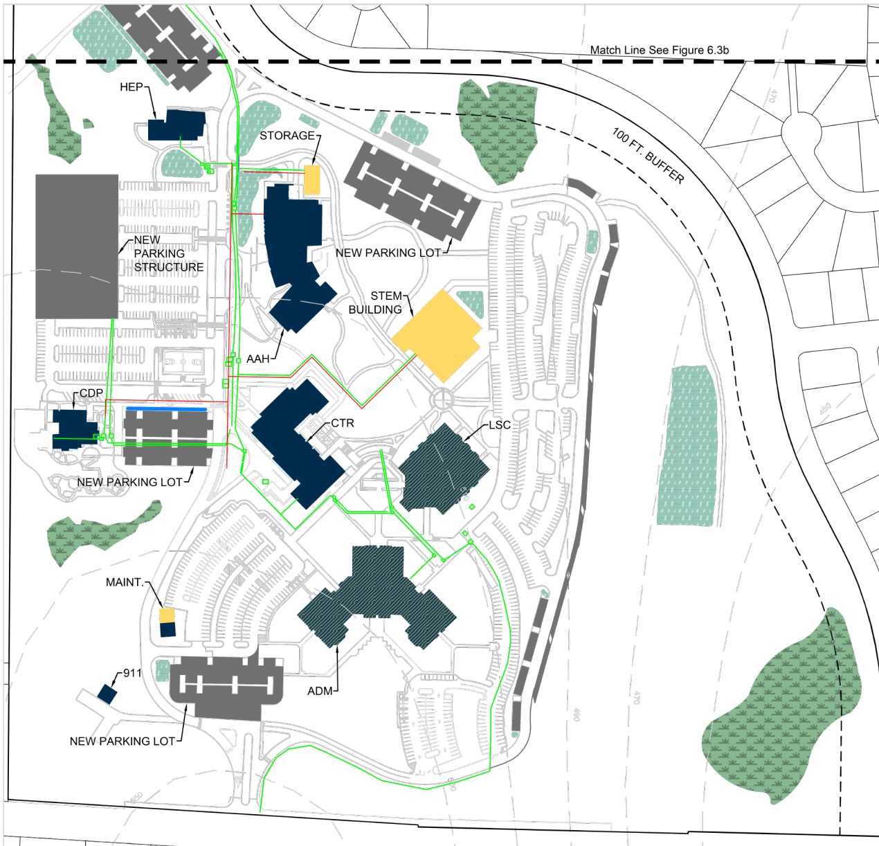
Figure 6.3a Power, Communications, and Gas Utilities
